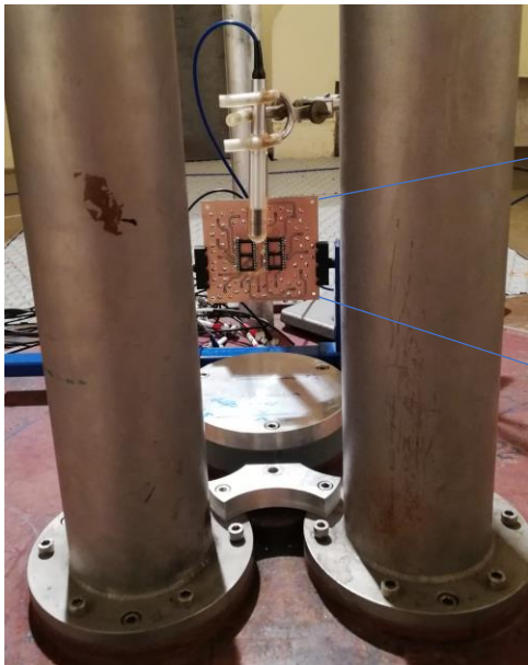
Two Cobalt 60 sources with a dose rate of 1.2 krad/h (Si).
